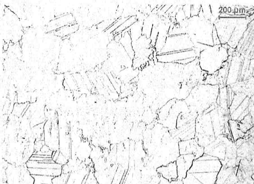
Figure 32. Microstructure of marble K. 1 year on the test wall. Plane-polarized light.
