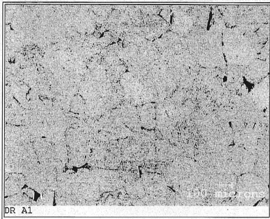
Figure 42. Marble D, 1 year on the test wall. BSE-image, 50x.
