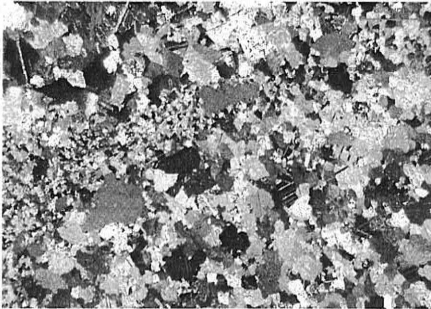
Figure 27. Microstructure of marble E. Unused. Cross-polarized light.
