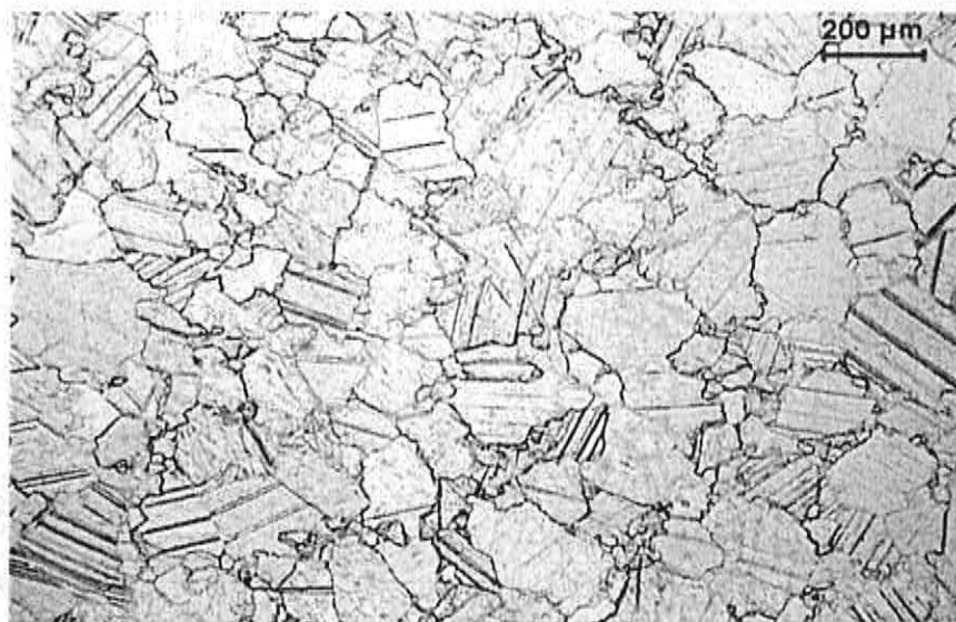
Figure 94. Microstructure of marble E(PA). Unused. Plane-polarised light.
