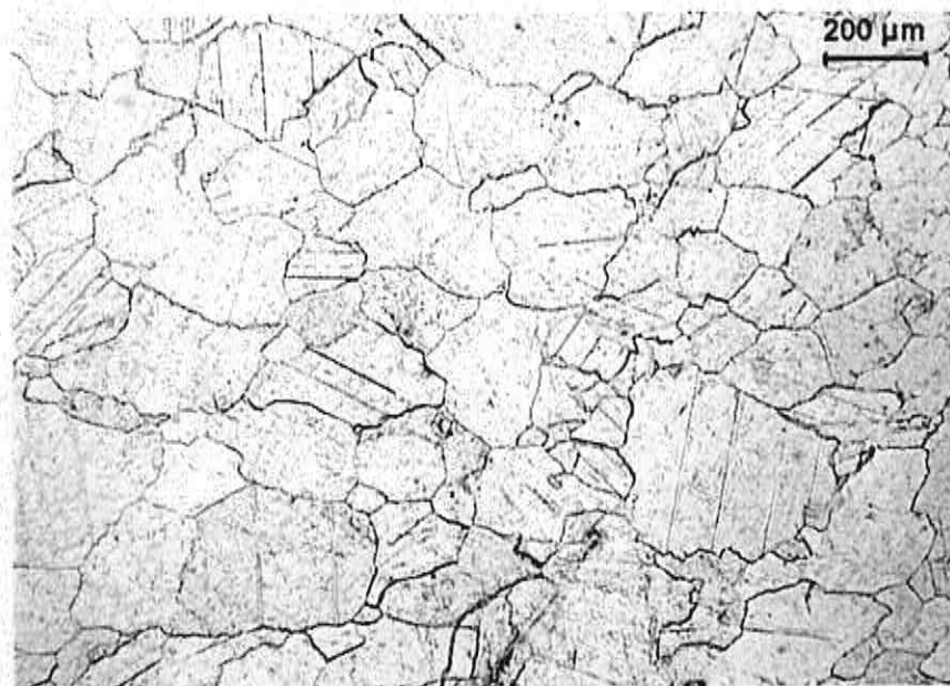
Figure 83. Microstructure of marble A protected with Prolapit. 1 year on the test wall. Plane-polarized light.
