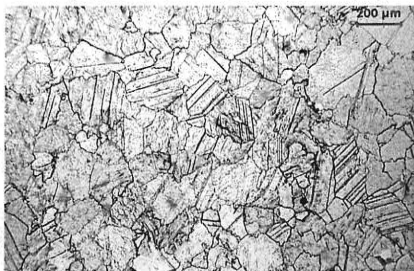
Figure 39. Microstructure of marble K. Unused. Plane-polarized light.
