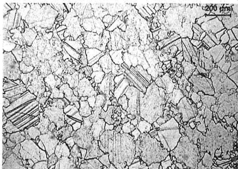
Figure 38. Microstructure of marble E. 1 year on the test wall. Plane-polarized light.
