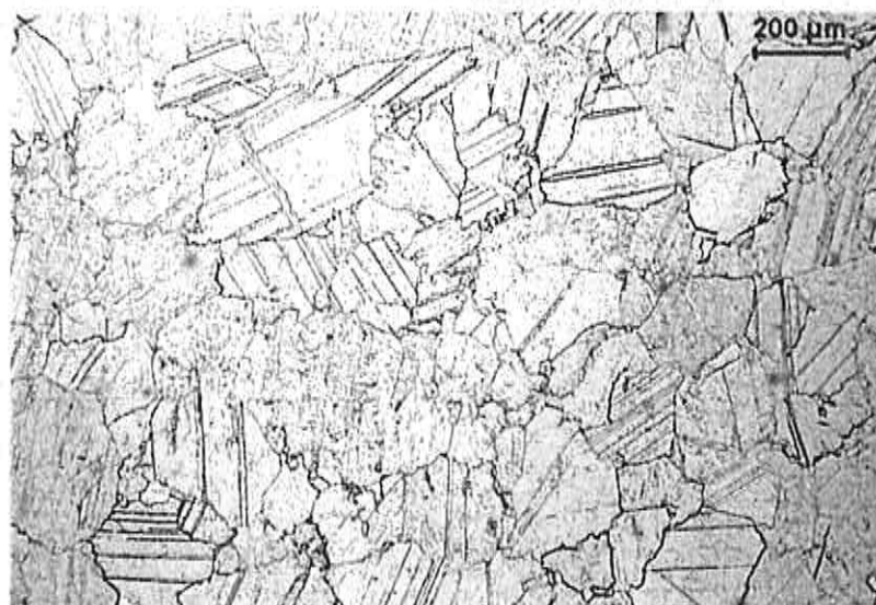
Figure 40. Microstructure of marble K. 1 year on the test wall. Plane-polarized light.
