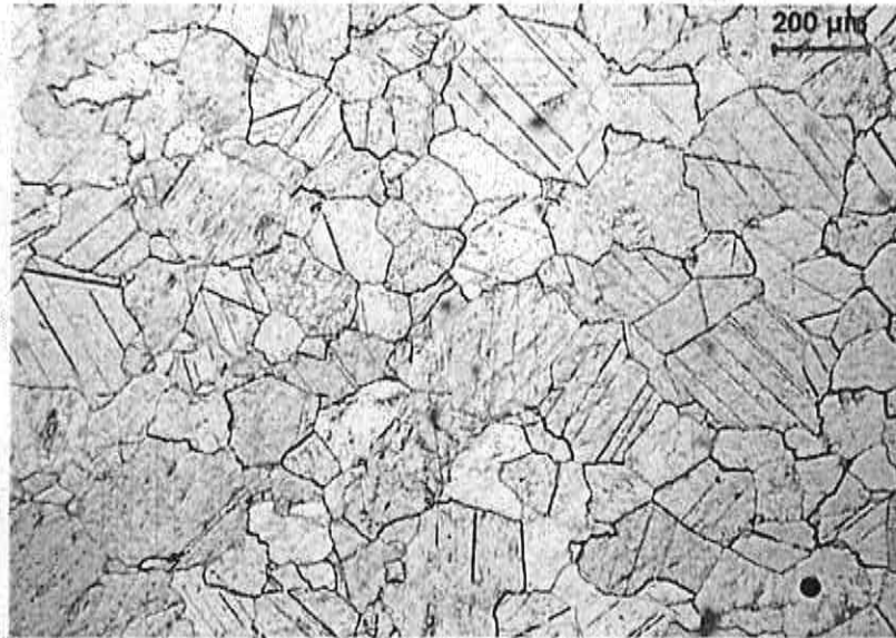
Figure 34. Microstructure of marble A. 1 year on the test wall. Plane-polarized light.
