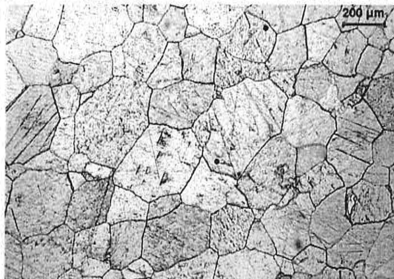
Figure 36. Microstructure of marble D. 1 year on the test wall. Plane-polarized light.
