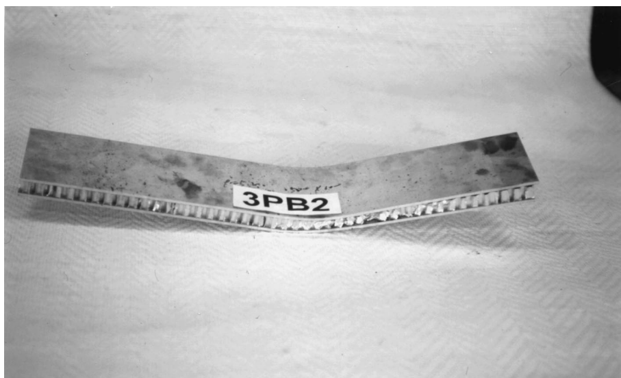
Fig. 6. Deformed shape of the specimen 3PB2 after testing.
