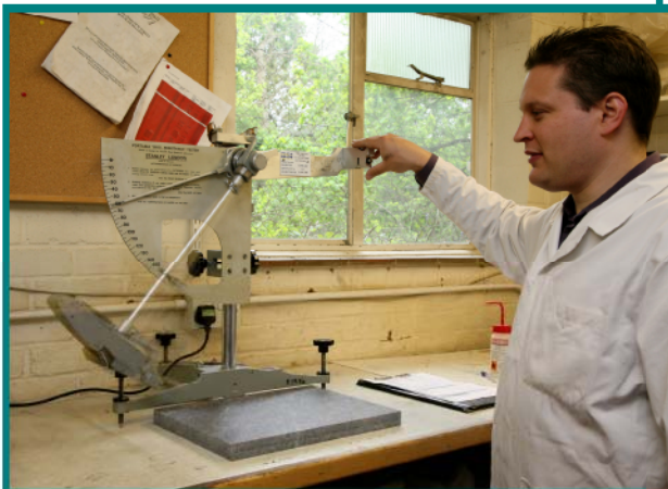
Pendulum slip testing in accordance with UKSRG
