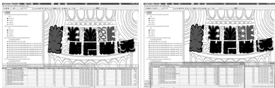
Figure 8. Cartographic attribution of CPI sets into the spatial entities of the thematic map of conservation interventions' planning (left). Spatial entity of the cleaning intervention of ion exchange resin with (NH 4 ) 2 CO 3 applied for 10 min, when CPI value changes from 8.14 (cross-hatched area in this Figure left) to 6.5 (dark grey area in this Figure right).
