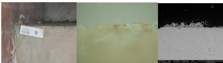
Fig. 6. a) sample 9 from a sound area, b) cross-section at OM, c) cross section at ESEM. In cross section no micro-cracks are visible indicating that marble is in good condition, not weathered.
