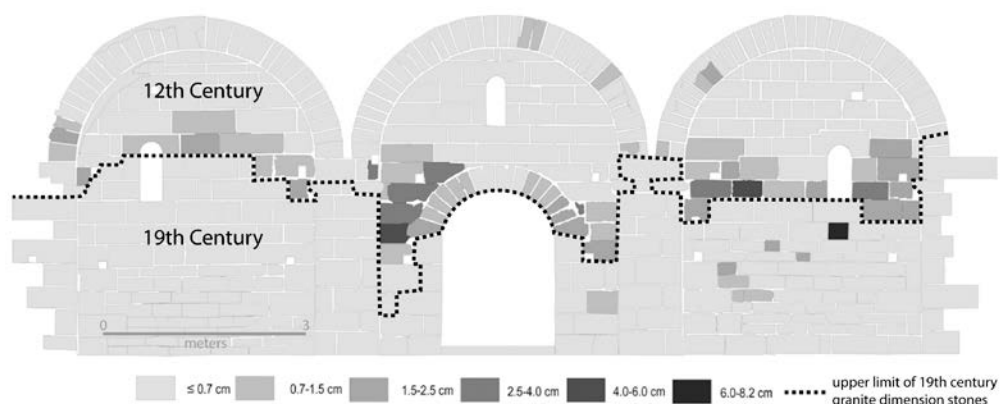
Figure 5. Accelerated stone recession just above the underpinned part of the arches based on 3D-modeling of stone decay by laser scanning. © Olivier Voldoire / Franck Vautier
