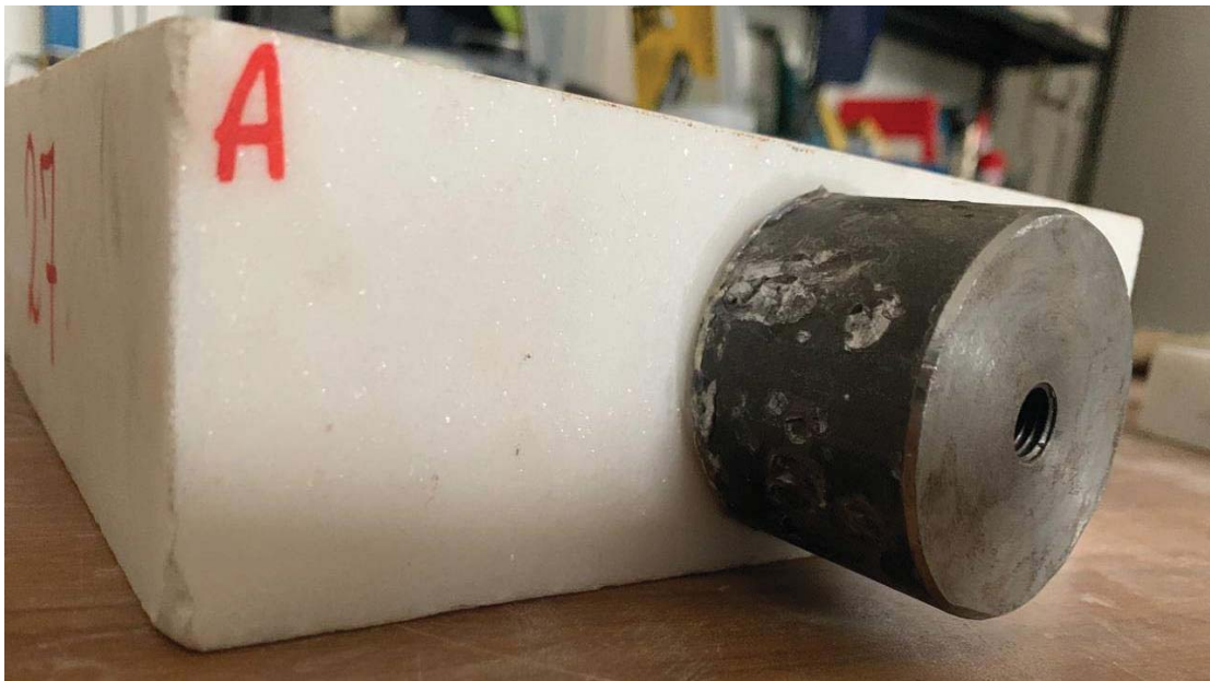
Figure 13 - Dry shear test configuration
