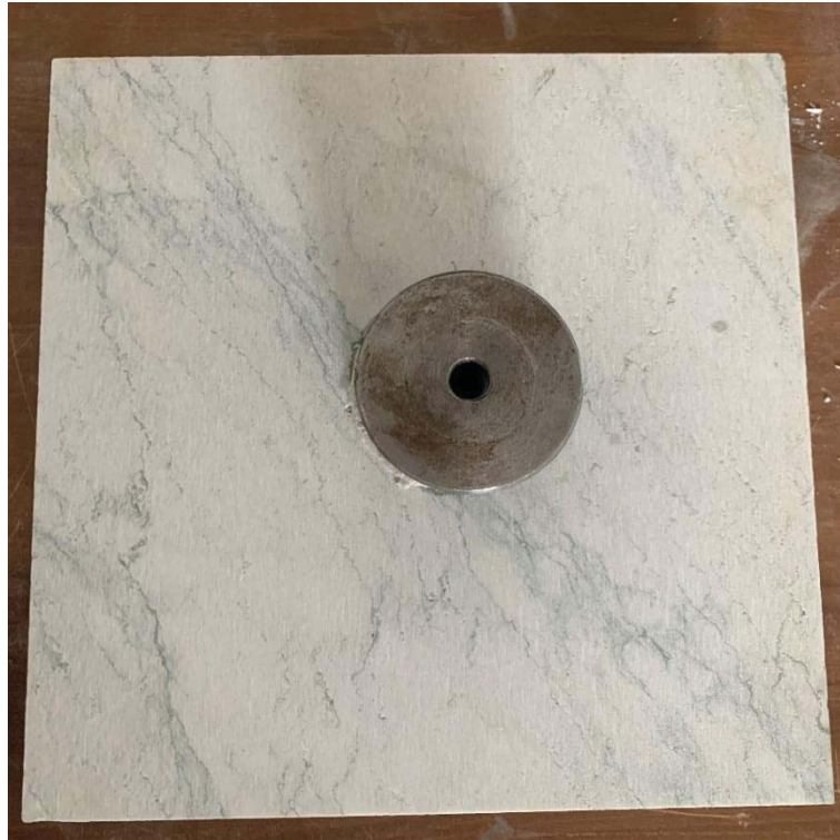
Figure 9 - Dry traction test configuration
