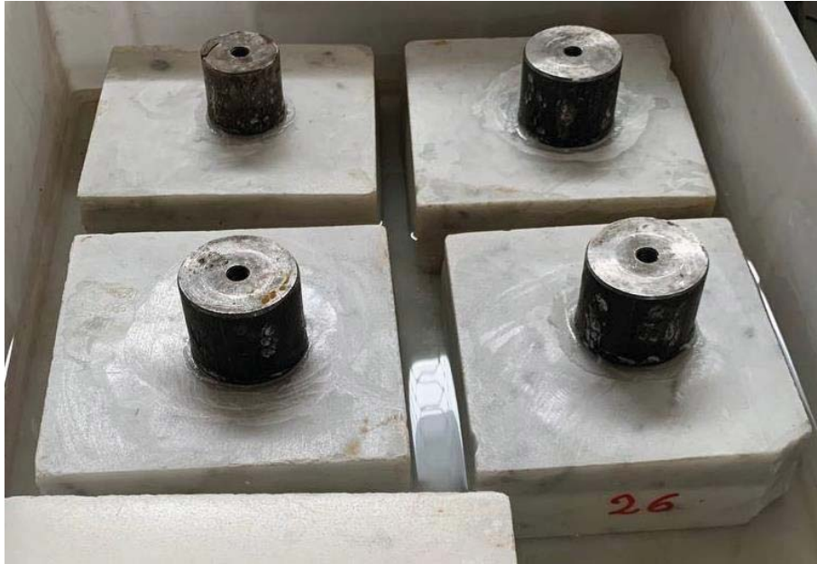
Figure 12 – “Wet 3” traction test configuration
