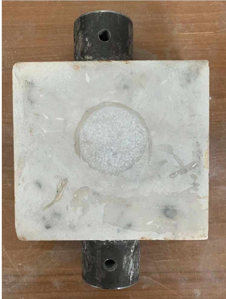
Figure 14 - Dry shear test configuration
