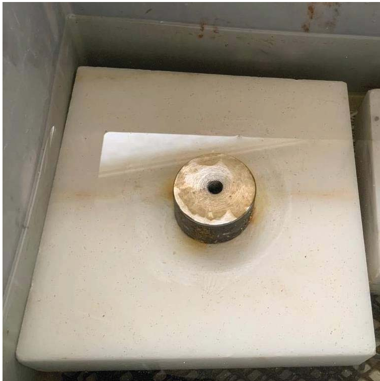
Figure 11 – “Wet 2” traction test configuration
