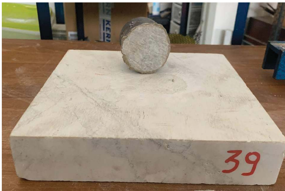
Figure 19 - Cohesive failure between adhesive and substrate
