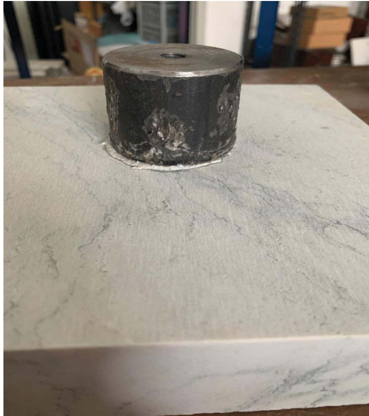
Figure 10 – Dry traction test configuration
