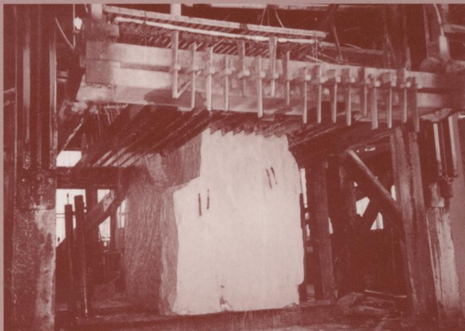
Marble quarry block is being sawed into slabs for use on a building façade
