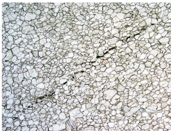
Advanced granular decohesion in white Gioia marble. As shown, the alignment of small-scale fractures (microfractures) produces an intergranular defect visible to the naked eye.
