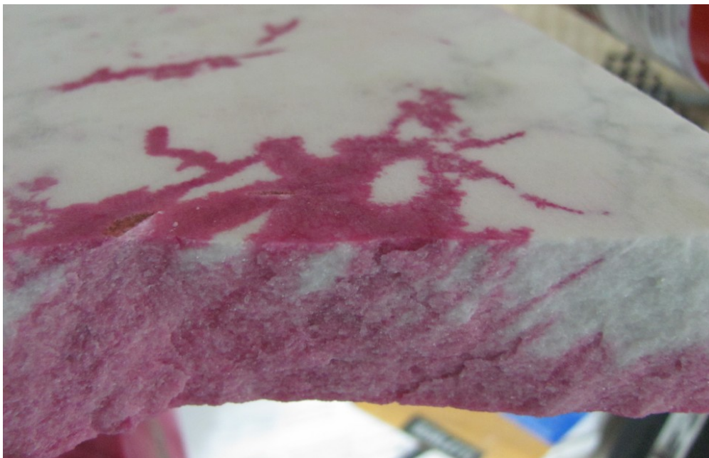
Lower face: the penetrant reached this face by following the verso direction.
