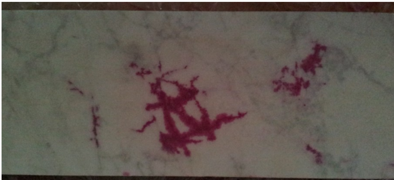
Lower face: the penetrant appeared along the pattern of the verso.
