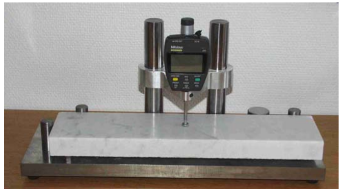
Figure 5. Measuring bowing in the laboratory.
