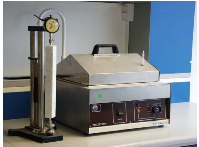
Figure 10. Expansion test-setup (right) and measurement of the length of the specimen (left).
